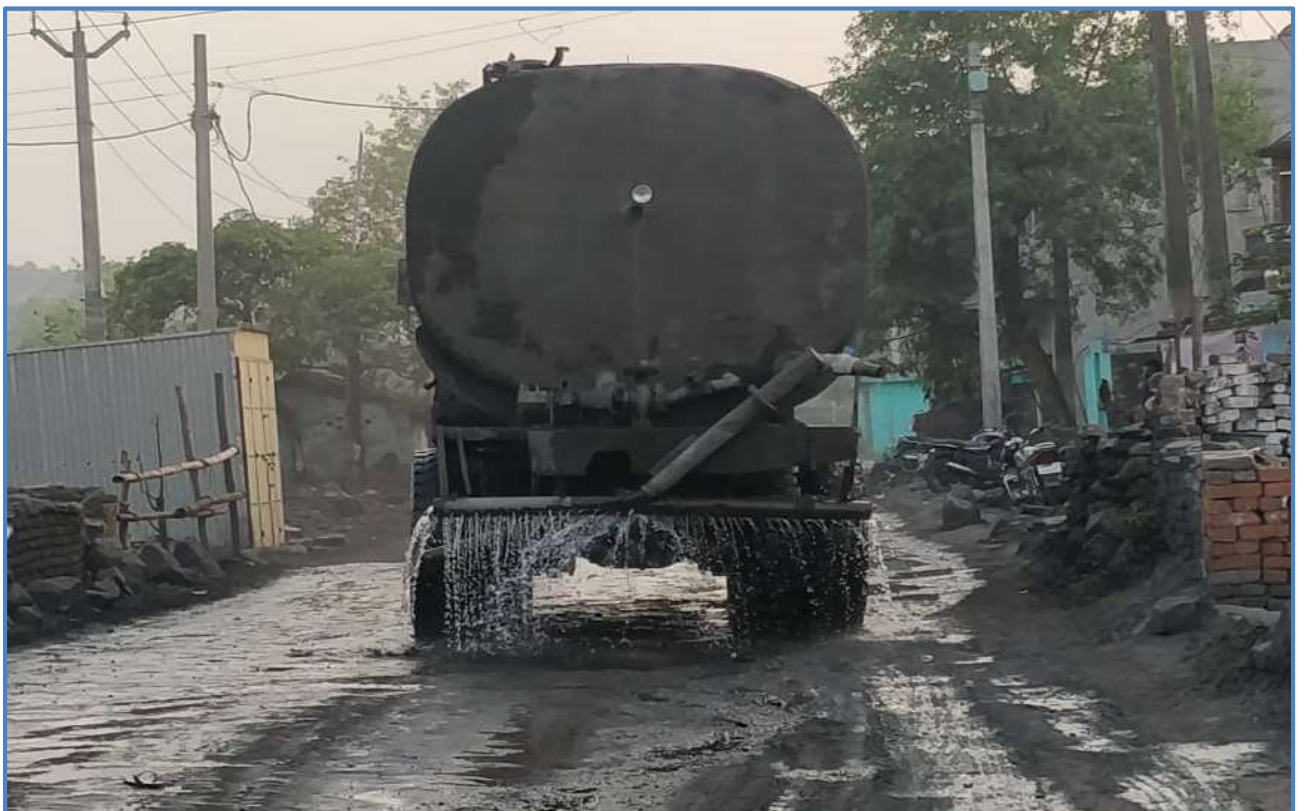
Picture 2 – Water Sprinkling on Transportation Road
